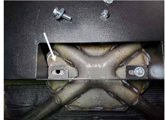
Attach forward section of mounting base to OEM cross brace using (2) 3/8" x 1" bolts, washers, and nylock nuts.
