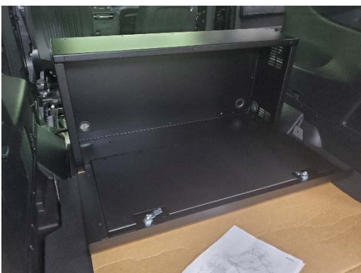
Slide the SBX-101 box into the rear of vehicle and rest on base.
