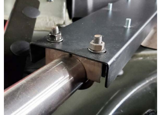
Attach other end of lower support bracket with supplied U-bolt, flat washers, lock washers and nuts. Repeat for other side
