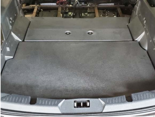
Remove forward section of the OEM trunk floor. T-55 Torx socket
