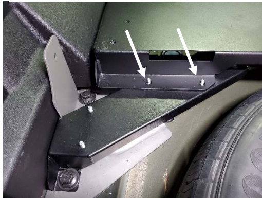
Line up to rear lower mounting brackets and attach using (4) 1/4" serrated nuts.
