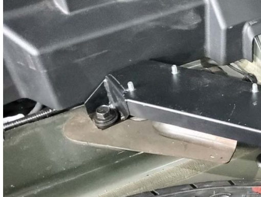
Remove rear bolt from OEM cross brace and install lower mounting bracket re-using OEM bolt. Repeat for passenger side
