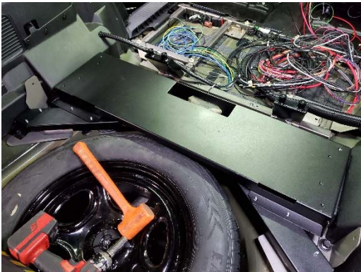
Place base into the rear of the vehicle.
